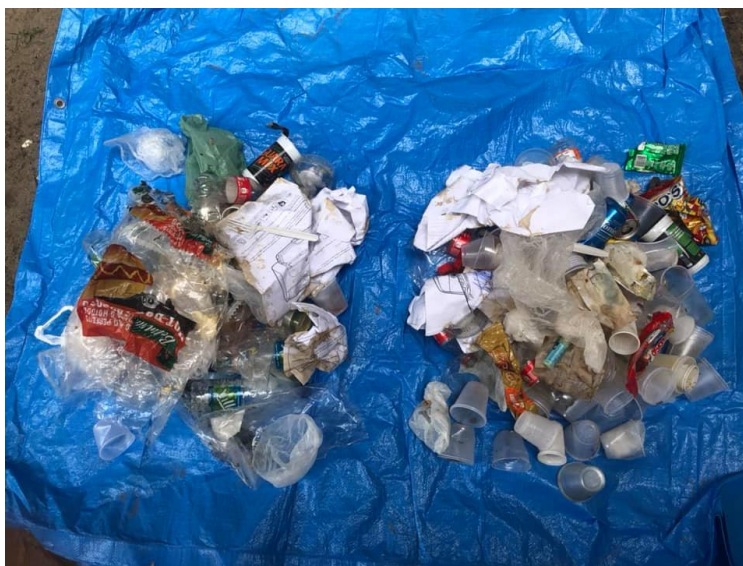
Figura 4: Processo de quarteamento (2/4 da amostra total). Figure 4: Quartering process (2/4 of the total sample).
